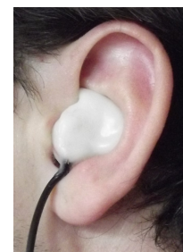
Fig. 2. Customized In-Ear PPG sensor to monitoring heart beat in left ear
